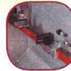
Bedknife mounts on permanent magnets with alignment stops and center supports.
