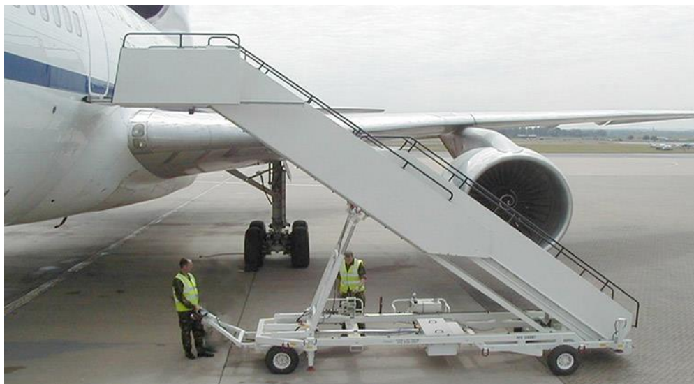
Example – Towable Aircraft Passenger Stairs
